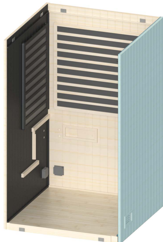
Figure 8. Installing Right Wall Section
