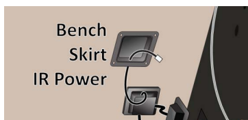
Figure 12. Bench Skirt IR Power Cable
