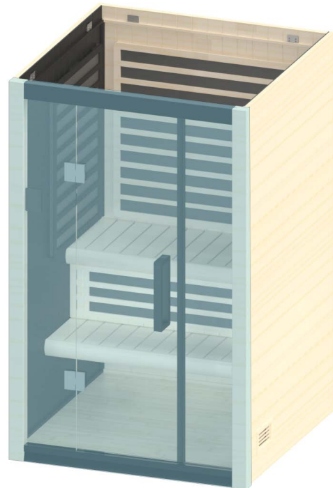
Figure 17. Installing Front Wall
