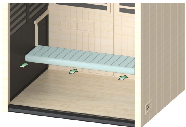
Figure 11. Installing Lower Bench
