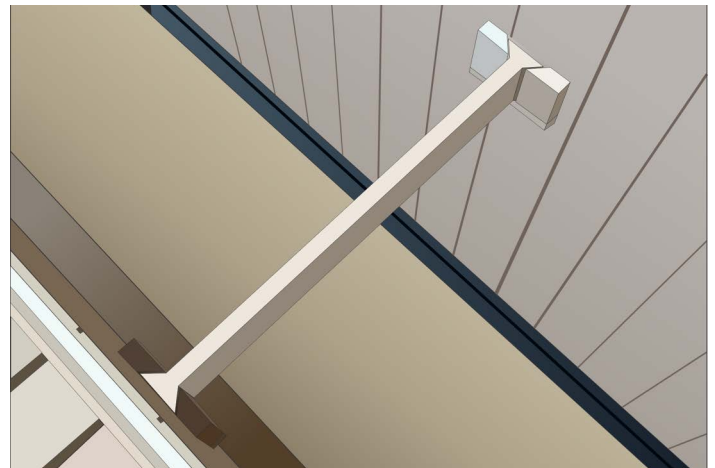
Figure 13. Installing Skirt Support Brace
