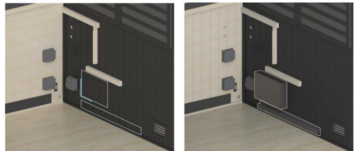
Figure 7. Mounting the CB Box to the Wall
