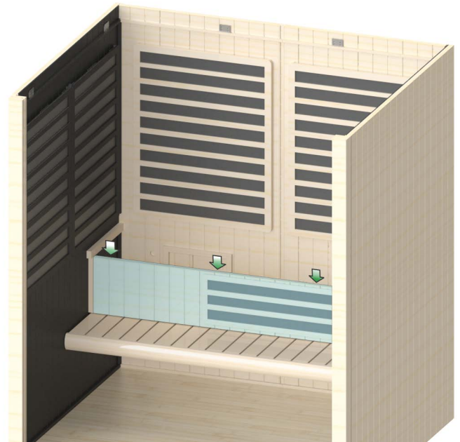
Figure 12. Installing Bench Skirt
