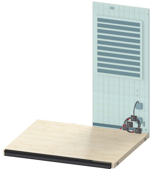
Figure 3. Installing Back Right Wall Section
