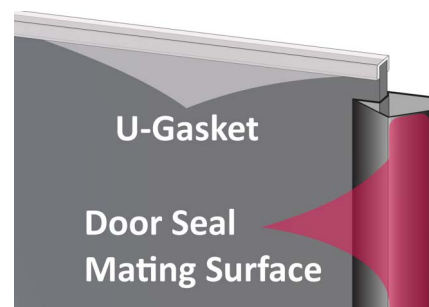
Figure 17. Single Glass Pane Orientation & U-Gasket
