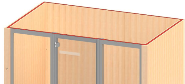
Figure 16. Applying Weather Stripping
