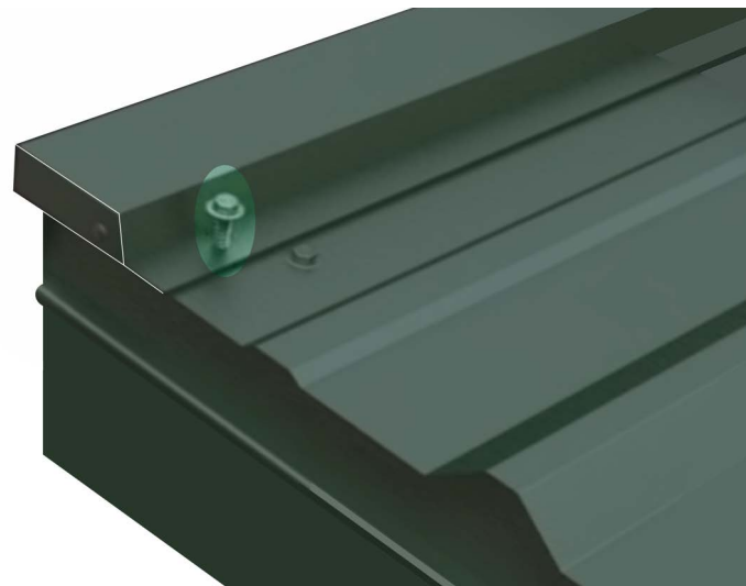
Figure 50. Attaching the Side Fascia
