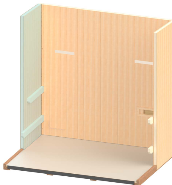
Figure 9. Installing Left-Back Wall Section
