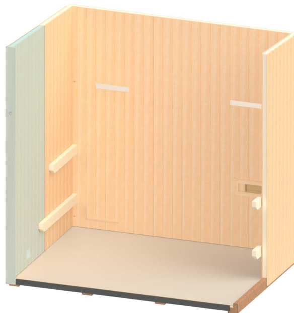
Figure 10. Installing Left-Front Wall Section
