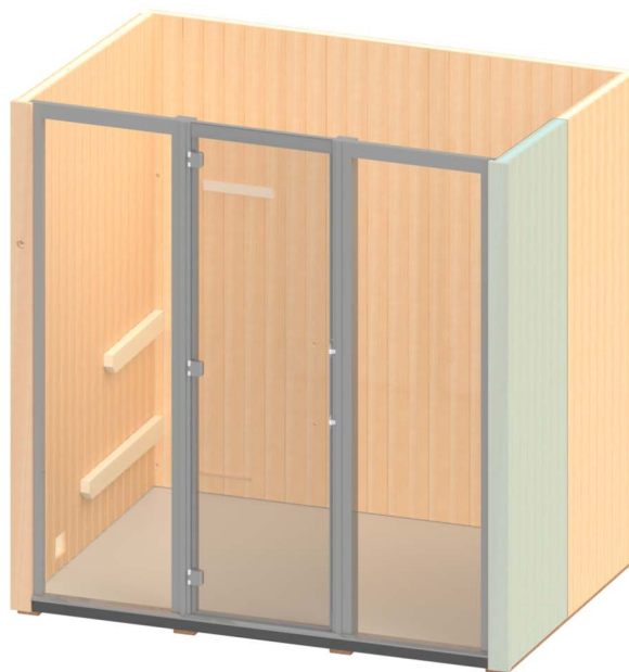
Figure 12. Installing Right-Front Wall Section
