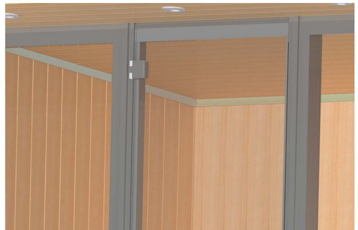
Figure 26. Installing Interior Cove Trim
