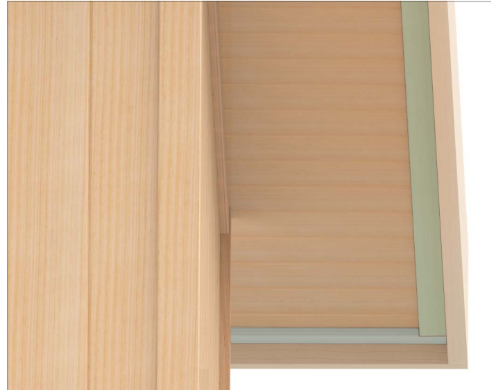
Figure 24. Installing Soffit Trim
