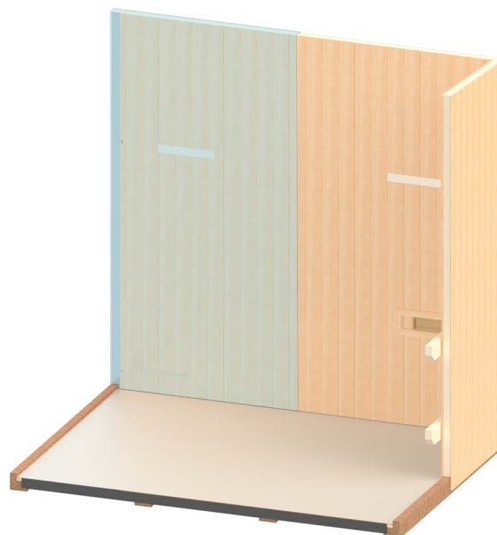
Figure 8. Installing Back-Left Wall Section
