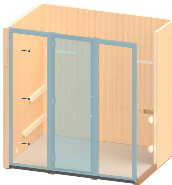
Figure 11. Installing Front Wall Frame Assembly
