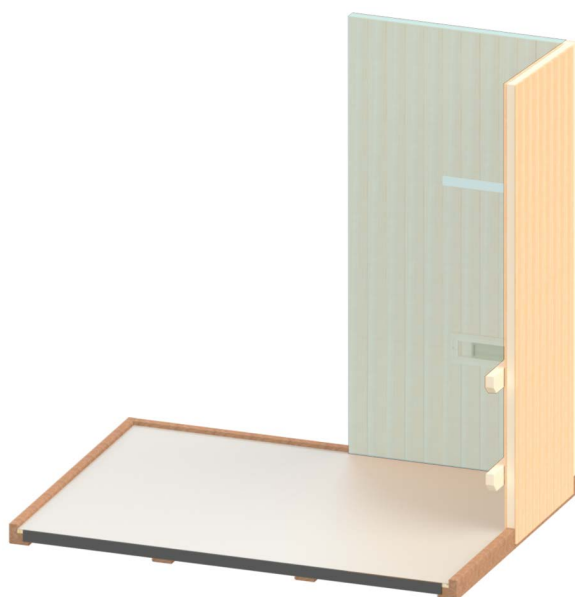
Figure 5. Installing #3 Wall Section
