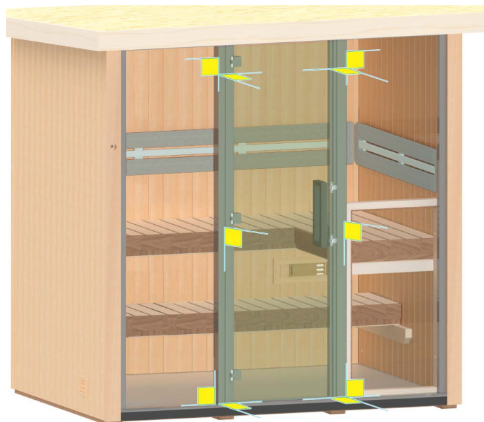
Figure 20. Aligning front wall frame Assembly
