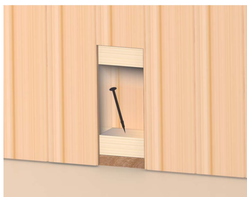
Figure 7. Pockets for Attaching Walls to Base Rail
