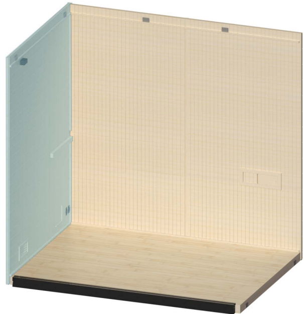
Figure 5. Installing Right Wall Section
