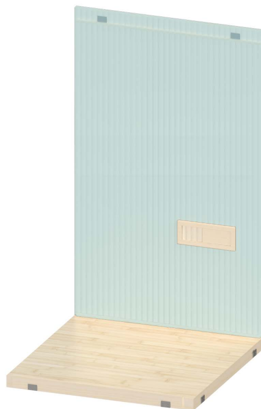
Figure 4. Installing Back Wall Section
