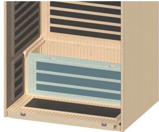
Figure 7. Installing Bench Skirt
