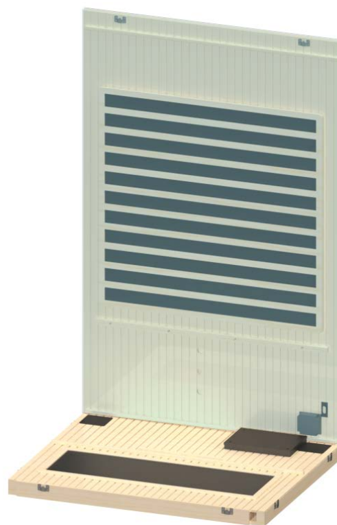
Figure 4. Installing Back Wall Section
